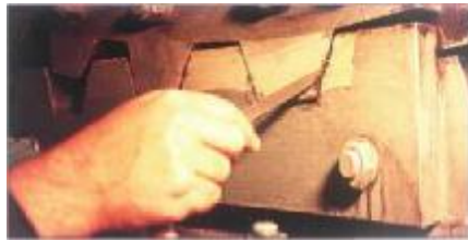
Fig. Measurement of flank clearance.
