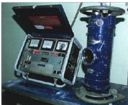
Fig. Control panel and x-ray tube.
