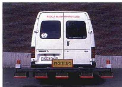
Fig. Survey vehicle with five radar antennae.
