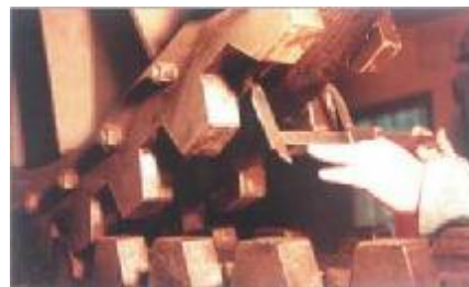
Fig. Measuring the width of the roller segment.
