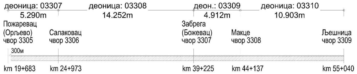
Figure 1-2 The length of the road section intended for rehabilitation (heavy maintenance)
